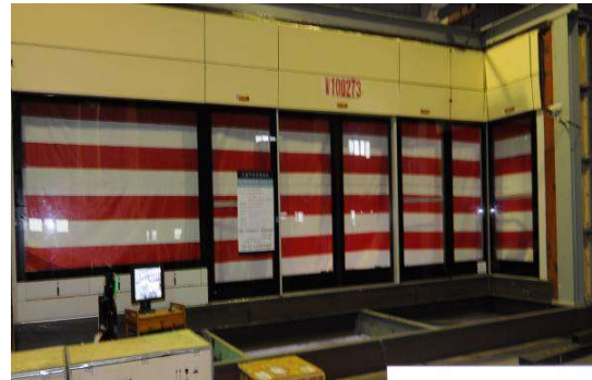
Endurability and Million Cycle Test for Platform Screen Door
