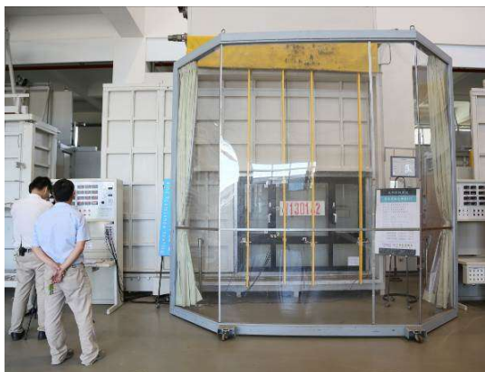
PVC safety shield used in Positive Pressure Performance Test
