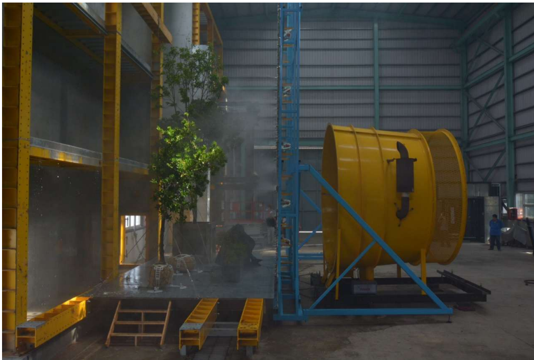
Dynamic Water Penetration Test with Plant in Progress at CT-380C
