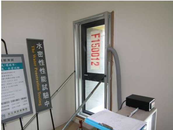
Field Water Penetration In Progress
