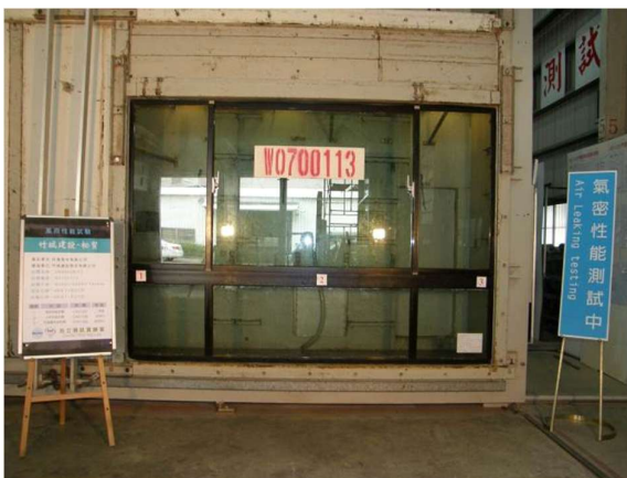
Air, Water and Pressure Test for Bottom Fixed Door and Upper Horizontal Sliding Window
