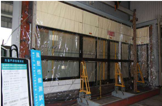
Positive Pressure Performance for Platform Scree Door in Progress
