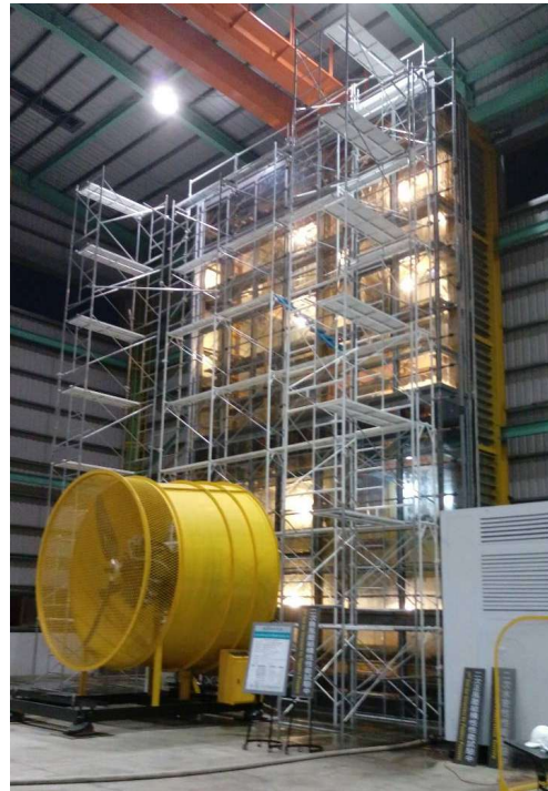
Front View of Curtain Wall Corner at CT-390C
