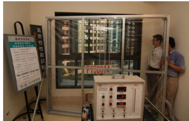
Open and Close Confirmation in Progress after Field Air Infiltration Test
