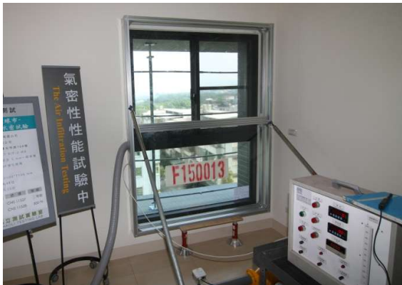
Field Air Infiltration Test in Progress
