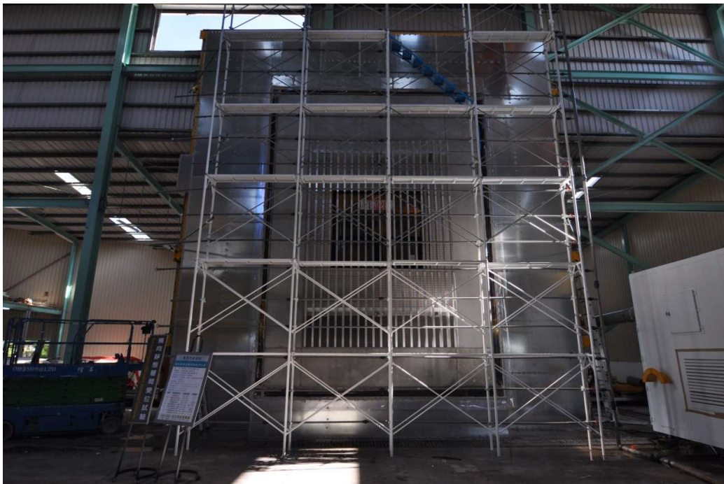
Interstory Displacement Test for Prefabricated Panel in Progress at CT-310C PC
