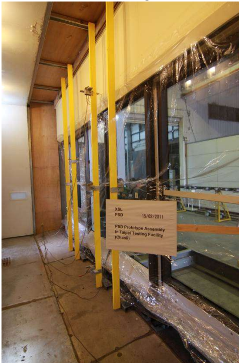
Retention Performance Test for Platform Screen Door in Progress
