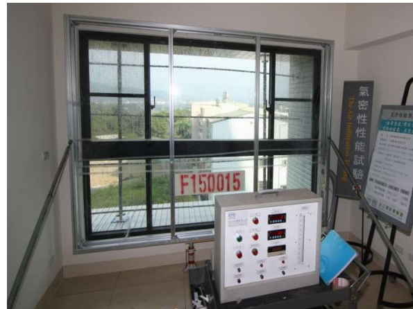
Air Infiltration Test in Progress
