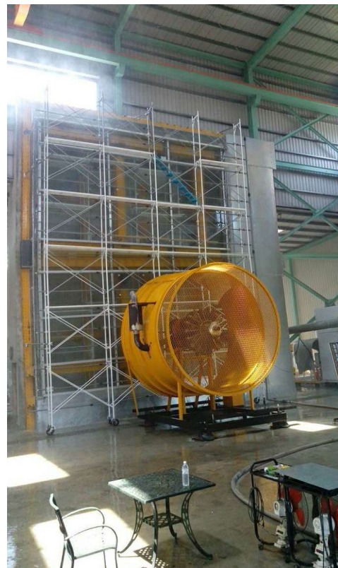
Test Completion of Curtain Wall Corner at CT-
