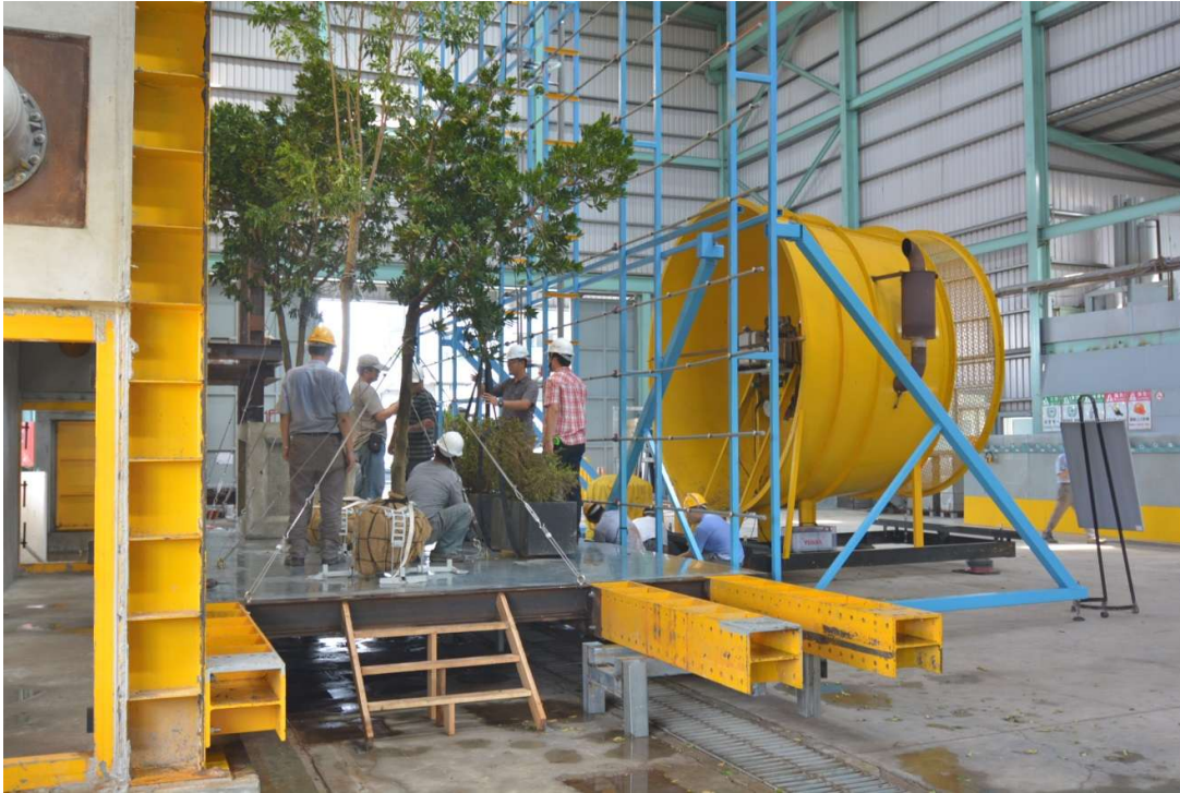
Planting Layout prior to Dynamic Water Penetration Test at CT-380C
