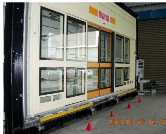
Air Infiltration Test for Platform
