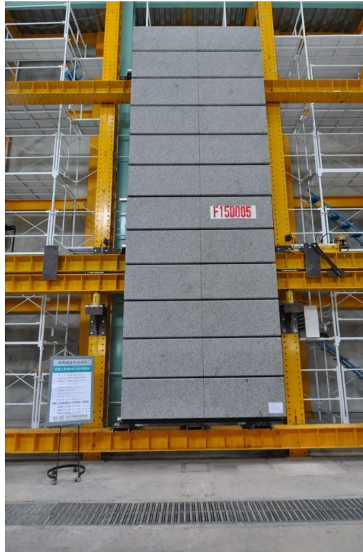
Interstory Displacement Test for Prefabricated Panel in Progress at CT-310C PC
